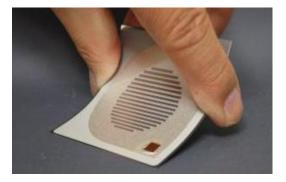
The thickness is about 1/4 of the standard ACM sensor and can be installed on curved surfaces such as inside and outside of pipes. The same lifespan and output as standard ACM sensors can be obtained.
